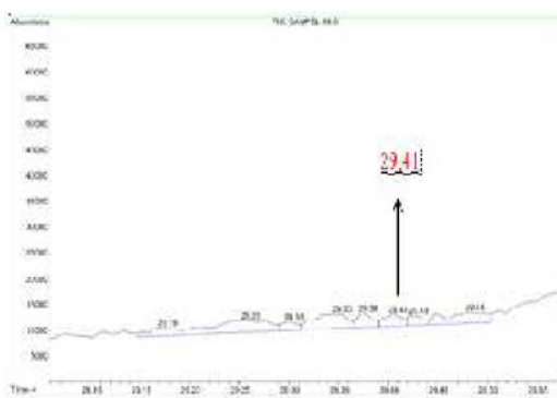
Figure 7. Chromatogram of phenanthrene in sediment samples after degradation with 0.07 M \text{KMnO}_4 , after the enlarged scale
